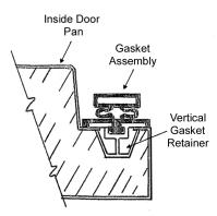
NOTE: The gasket may appear too large, but if it is installed as indicated above it will slip into place.
